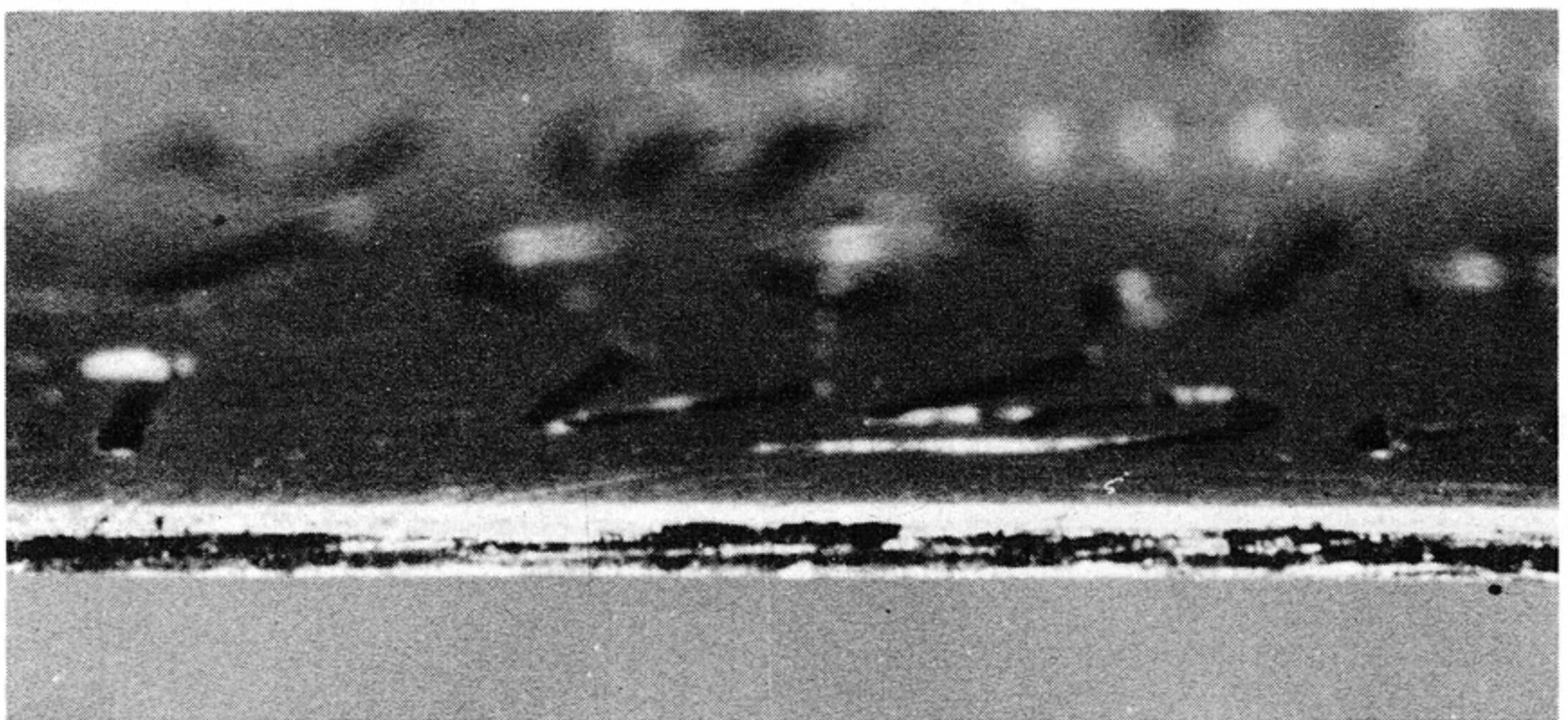
Figure 3. One edge of Plate 10 showing that it was filed to size. Note file marks running lengthwise on the edge.
