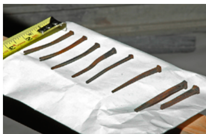
FIGURE 7. Cut nails removed during the 2006 renovation. Photograph by Arnold Angle.
